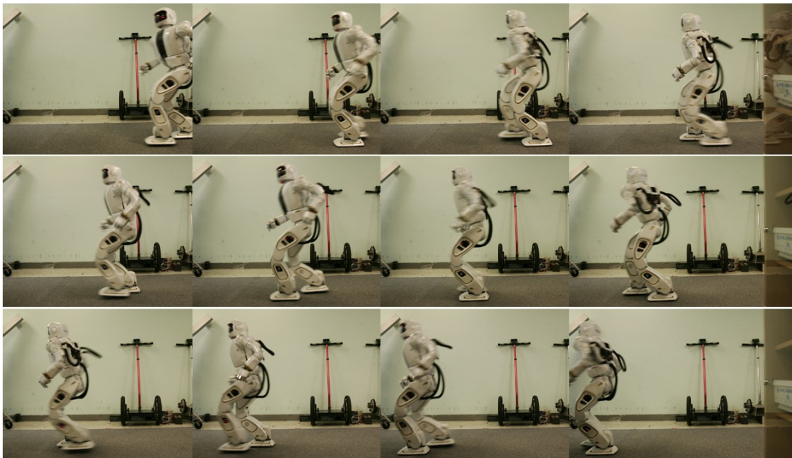
Figure 16. Photo sequence of the running experiment of HUBO2
